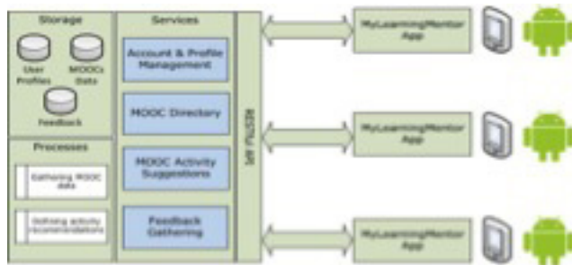
Figure 1. Diagram of MyLearningMentor architecture with the server on the left and the client on the right.
